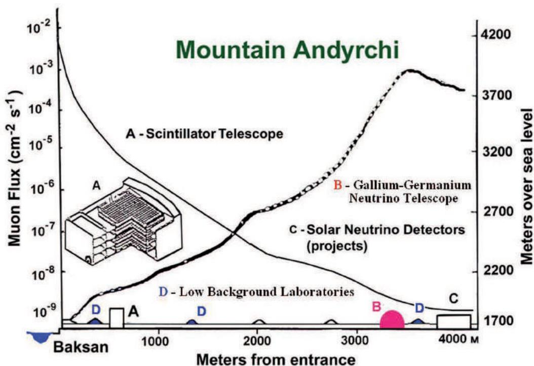
Fig. 6. Schematic view of a section of the Andyrchy slope along the adit (right scale) and dependence of underground muon flux on the laboratory location depth (left scale).
