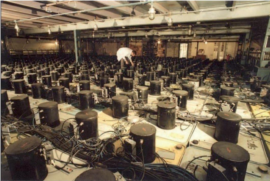
**Fig. 7.** A view of the BUST top horizontal plane.
