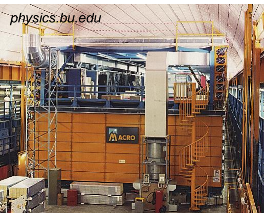
MACRO – 76.5 \times 12 \times 9.3 \text{ m}^3 , liquid scintillation counters, limited streamer tubes and nuclear track detectors
