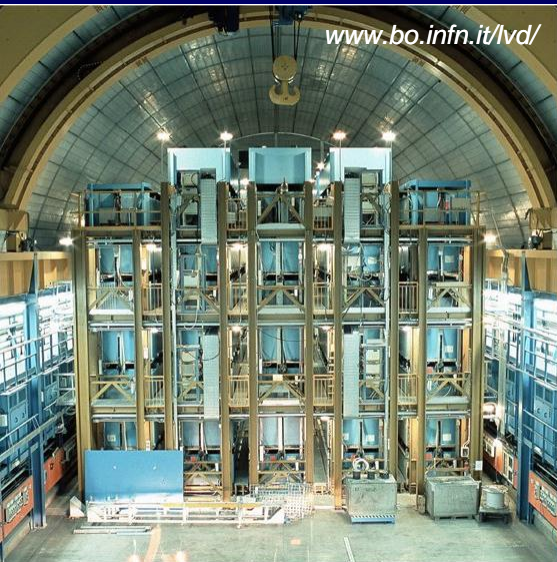
LVD – 840 liquid scintillation tanks 1 \times 1.5 \text{ m}^3 , streamer tubes modules
