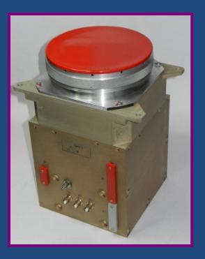
BDRG instrument consists of 3 similar detector boxes, connected to data analysis box.
